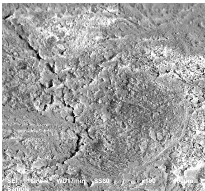
Figure 6. SEM image showing cracks present on the surface of the mortar.
