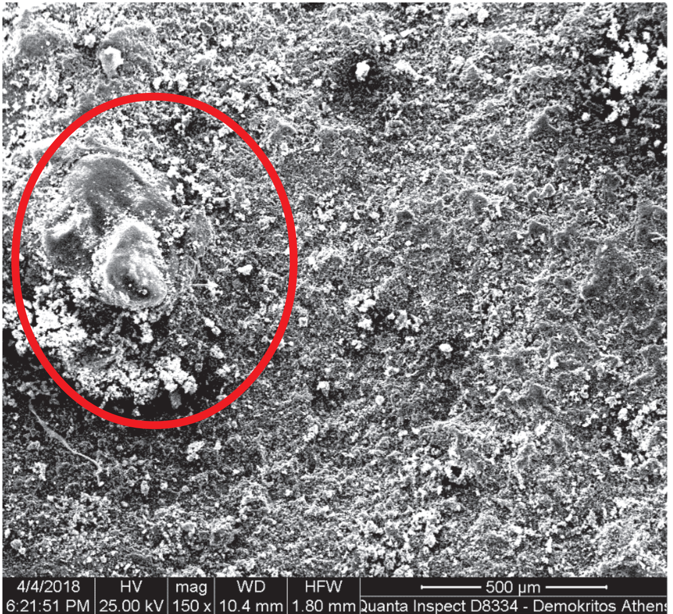
Figure 8. SEM image showing the presence of the white layer on mortar surface.
